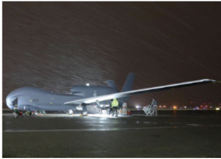
RQ-4B maintenance crews make Pre-Flight inspection for the night mission
