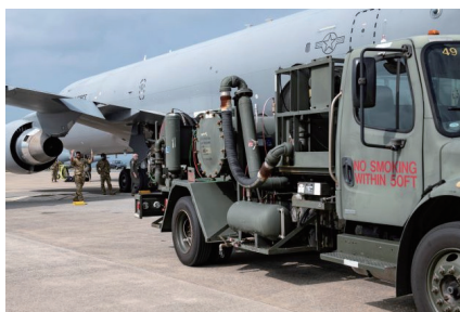
An Airman from the 22nd Air Refueling Wing marshals an R-12 refueling truck into position for hot pit refueling operations
