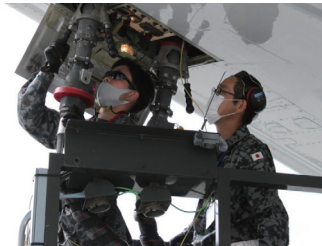
Two Koku-Jieitai maintenance specialists refuel an E-767 from USAF tank truck in JBER
