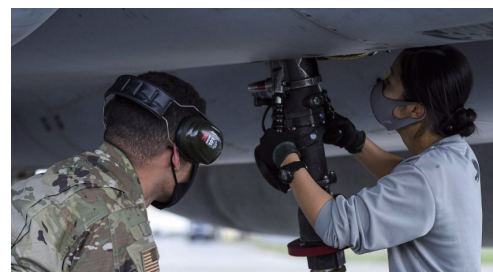
A Koku-Jieitai maintenance specialist refuels a F-15 from USAF tank truck in Eielson AFB
